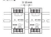
When installing multiple SMPSs, please keep space at least 10 mm between SMPSs for heat radiation
