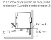
• When mounting this unit on the rail, place the unit at least 30 mm above from the floor to remove it easily.
