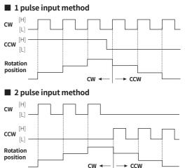
• Do not input CW, CCW signal at the same time in 2 pulse input method.
